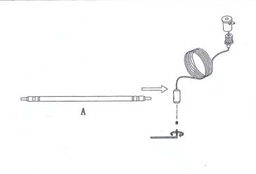
Connector A inserts in pendant assembly, to the right position. Then fasten the screw.
