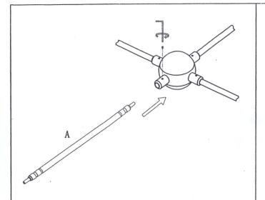
Connector A inserts in balls, and fasten the screw.
